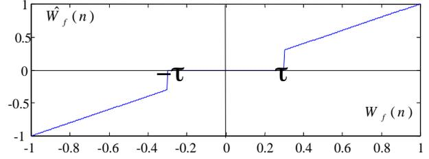
Figure 3: Hard thresholding rule.
