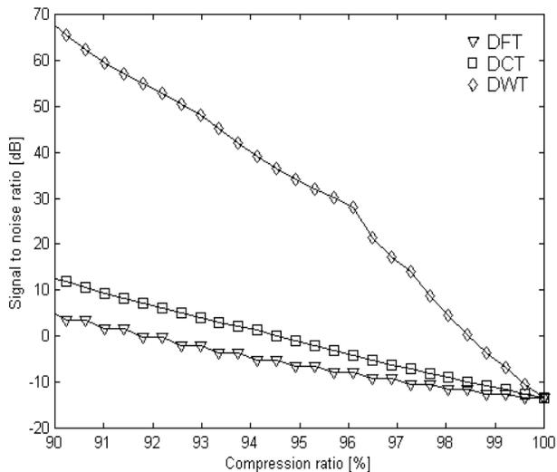
Figure 4 – Compression ratio performance with experimental data
